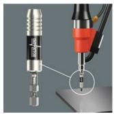
The Impaktor stainless steel holder with a retaining ring and magnet satisfies the extreme, dynamic requirements in that there are consciously no small mechanical component parts fitted as they would be more susceptible to failure. It focuses on the basic bit holding function and the cushioning of the extreme impulse peaks with its two different torsion zones. Mainly used in industrial screw assembly applications e.g. with screwdriving robots.
